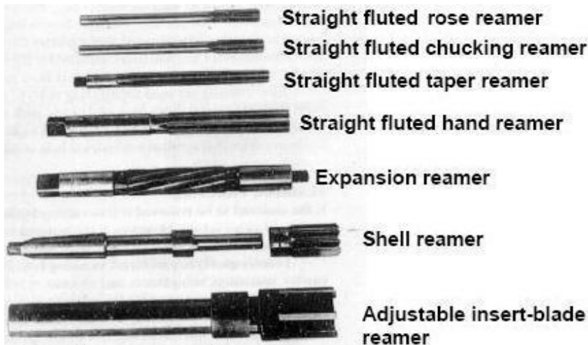
Fig. Different types of reamers
